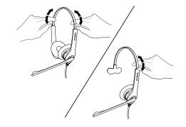
Jabra Biz 1500 has a 270° boom arm so it can be easily adjusted without breaking.
