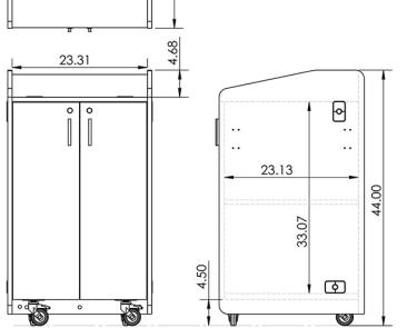
The lectern model **LE3050** is a mobile lectern with a convenient flat top surface to accommodate lecture notes, laptops or monitors. The lockable lower cabinet has an adjustable shelf and ample storage space for your presentation media, microphone and other electronic equipment, etc.
